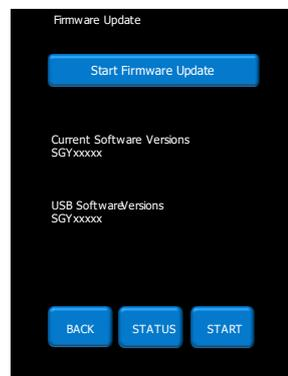
**ENSURE POWER IS NOT REMOVED FROM THE UNIT DURING THE FIRMWARE UPDATE**
