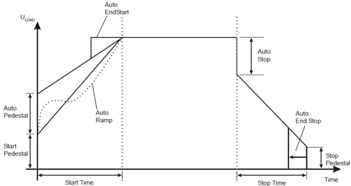
**Automatic Pedestal** - Automatic overriding of the start pedestal. When On the unit approximately detects the start of motor rotation and tries to adjust the pedestal to suit.
