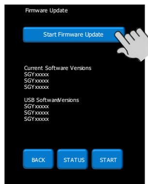
**ENSURE POWER IS NOT REMOVED FROM THE UNIT DURING THE FIRMWARE UPDATE**
