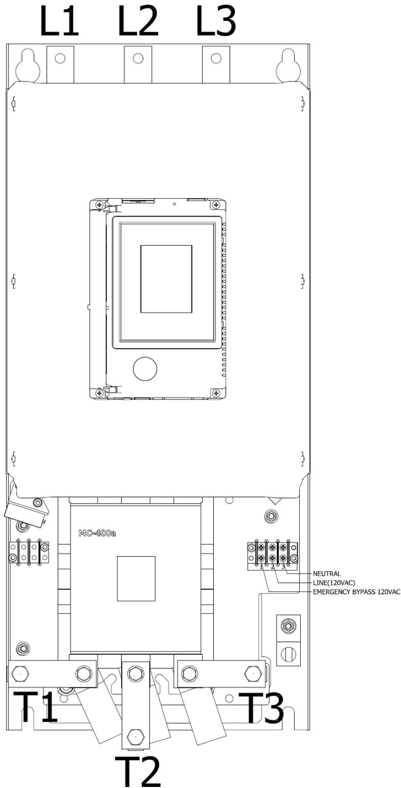
Supply 120 VAC control power to terminal 2 and 3 of the 120 VAC control power terminal block shown above. To close the contactor for Emergency purposes put a jumper between terminal 1 to 2 or supply 120 VAC to terminal 1 and 3.”
