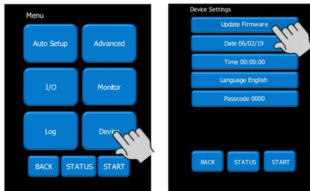
3. The next screen shows the 'current' installed firmware version and the firmware version previously copied to the USB flash drive. Press the Start Firmware Update button. Confirm the update
