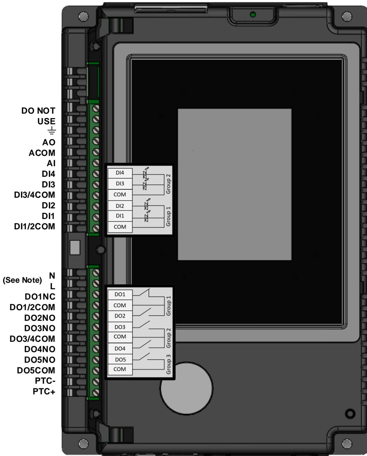
**NOTE:** AC Input terminals L & N on starter module only available on models VMX-SGY-A-18 to VMX-SGY-A-160. For all other models the control power input is located on the chassis frame mounted terminal block.
