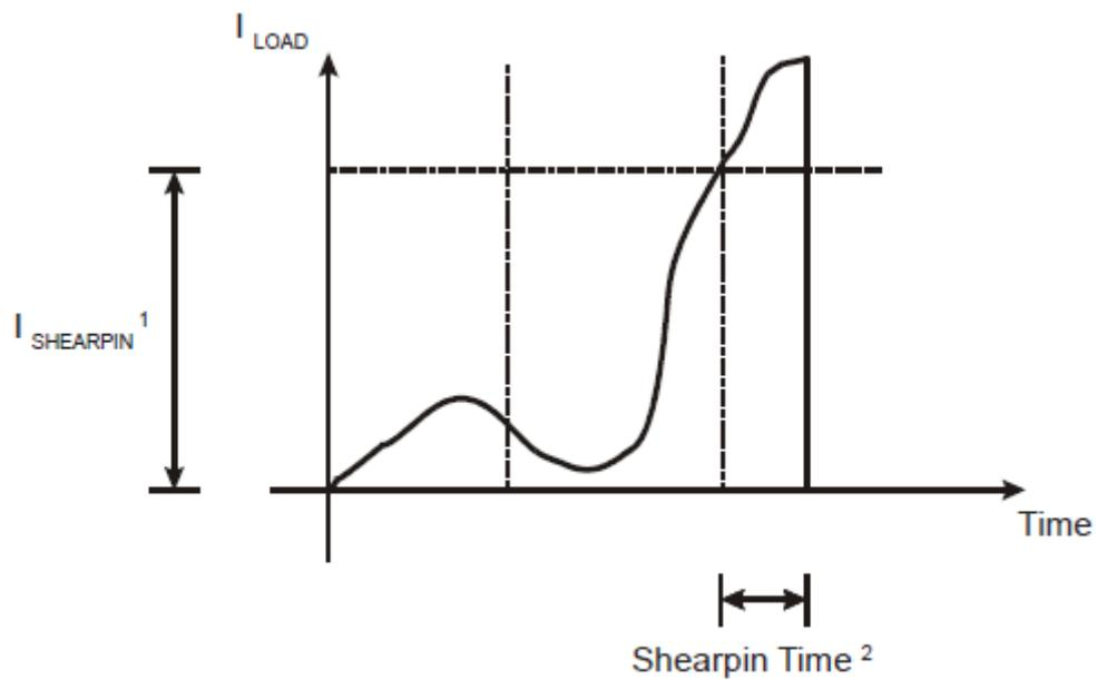
1.  $I_{SHEARPIN}$  = Shearpin Level.
