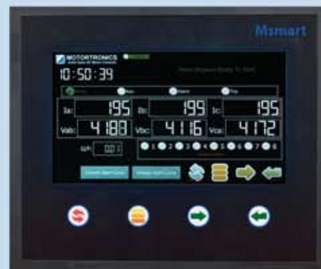
Msmart is a single interface to commission, start-up and diagnose the MVC4 and auxiliary devices.
